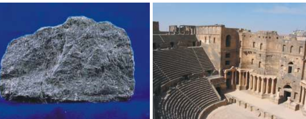
Fig.3 Typical basalt stone and the Roman theatre in Bosra, Syria; the dark building stone is basalt.
