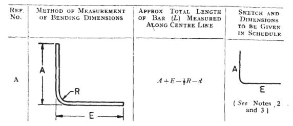
As per above table V of IS 2502, cutting length of bend and 2 half legs L = A+E - (R/2)-d. Thus the total length of a bend, and respective 2 half sides = (L/2 + W/2-R/2-d)) Will be = ((600-80)/2) + ((400-80)/2) - (4\*10/2)-10} = 390mm
