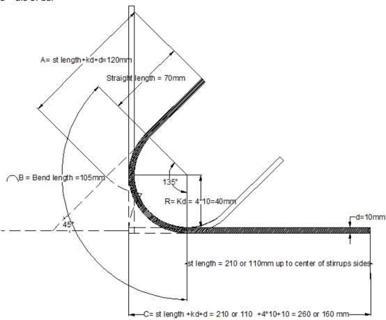
If we consider C = half length of stirrups side then it will be 210mm or 110mm +kd+d Cutting Length of hook + an half stirrups side will be = 175+210 and 175+110
