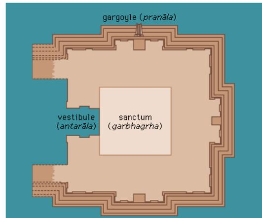
Fig.17c – Typical plan of Inner Chamber of an Indian Temple
