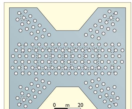
Figure 3. Layout of the 172 no. 2.5 m diameter bored piles and 5.5 m thick raft
