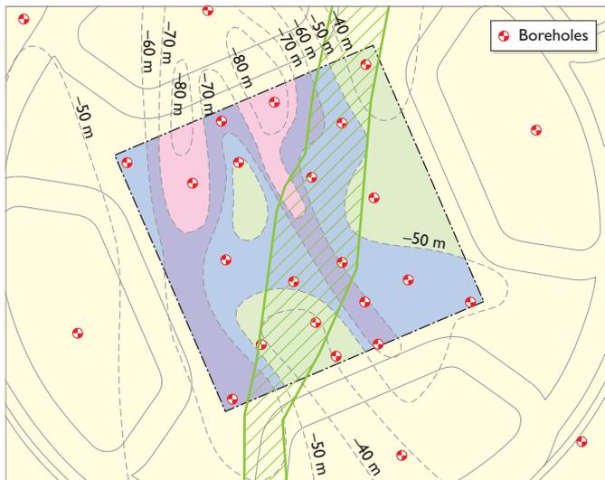
Figure 2. Borehole-derived contours of the soft rock surface under the Incheon Tower foundation – the depth varies from 40 to 80 m
