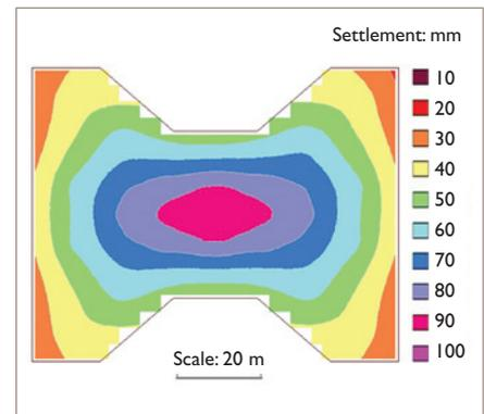
Figure 5. Typical set of computed settlement contours for the Incheon Tower
