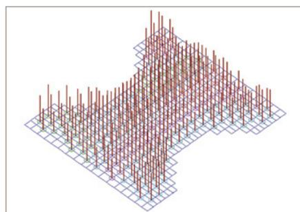
Figure 6. Computed distribution of axial pile loads for the Incheon Tower
