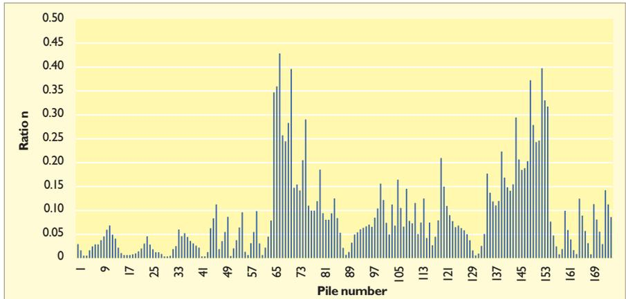
Figure 4. Assessed values of  $\eta$  for each pile from cyclic loading analysis using a load case 0.75 (dead load + live load + wind load)
